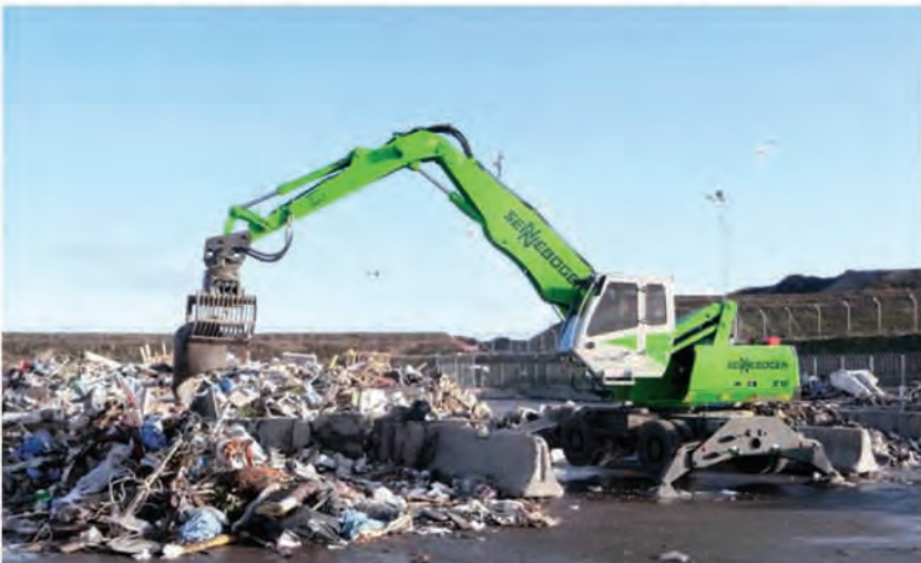
818 M – with sorting grab – sorting of waste; Sweden
