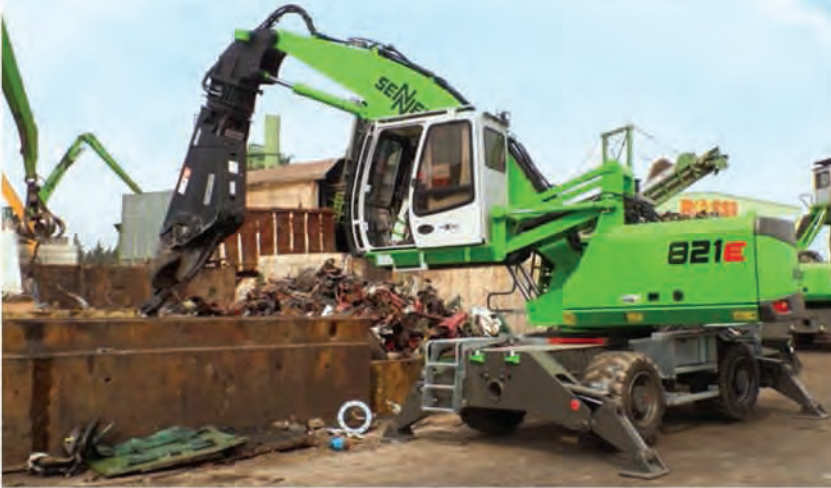
821 M – with 4 t scrap shear – shearing of scrap; France
