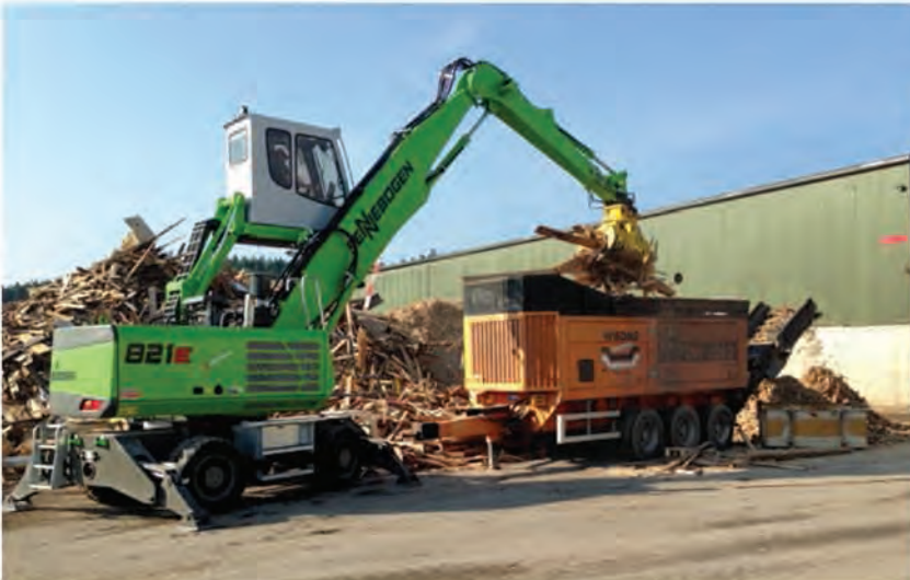
821 M – with sorting grab – feeding a shredder with used wood; Switzerland
